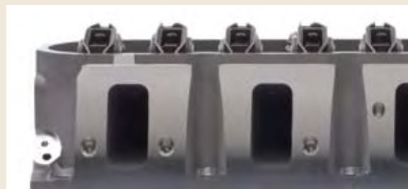
C L92 Intake Port and Bolt Pattern
